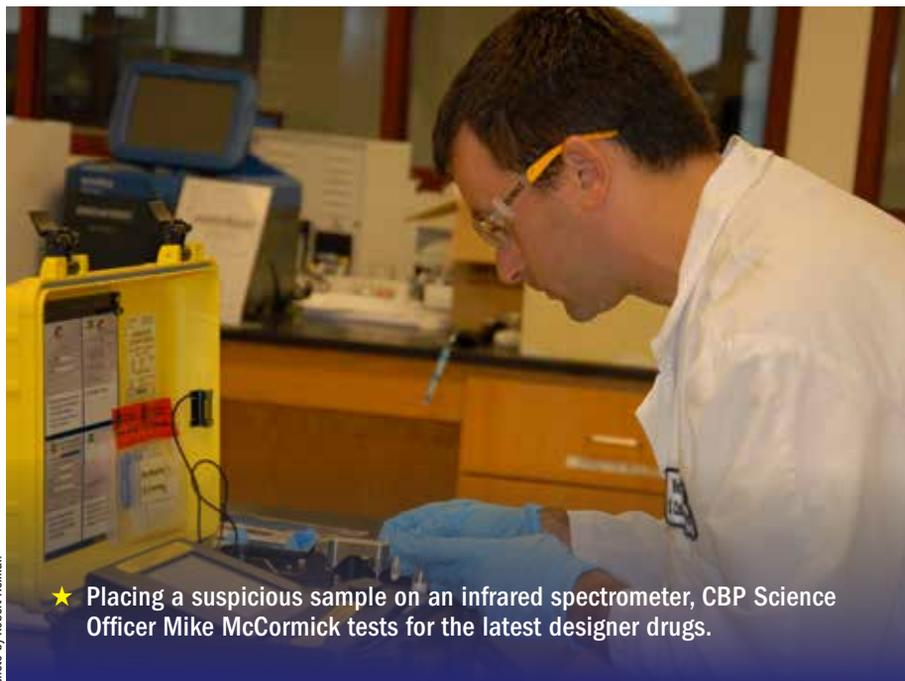
★ Placing a suspicious sample on an infrared spectrometer, CBP Science Officer Mike McCormick tests for the latest designer drugs.
